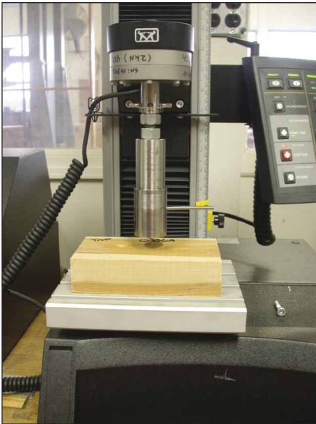
Figure 2—Modified Instron equipment for ASTM D 143 test of Janka hardness. Penetration depth of Douglas-fir 2×4 measured electronically.
